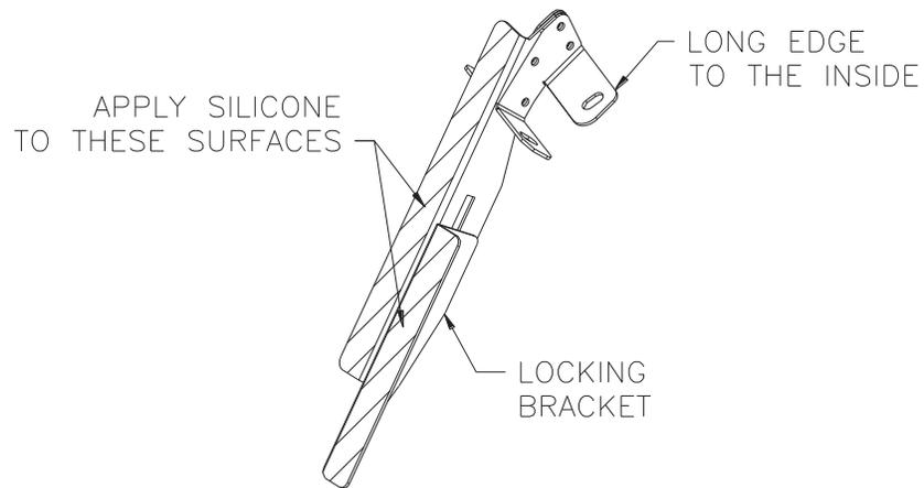
12. Re-install the sunvisor halves by hooking the outside bracket in the sunvisor notches, then fit between the center bracket halves. Extend the locking bracket into the lower notch and tighten the carriage bolts. Install the  $\frac{1}{4}$ -20x $\frac{3}{4}$ " hex bolts, washers and locknuts through the center bracket and sunvisor halves.
